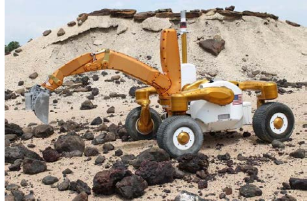
Fig. 1: Combination of JSC Centaur 2, GRC APEX, and Kennedy Space Center percussive bucket.
